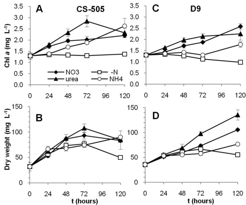
**Figure 2.4.1** Growth curves of *C. raciborskii* CS-505 (A, B) and *R. brookii* D9 (C, D). Curves were plotted by chlorophyll *a* and dry weight per unit culture volume. Values are shown as the average of three biological replicates; error bars indicate  $\pm$ SD from the mean ( $n = 3$ ).
