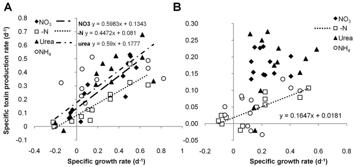
**Figure 2.4.S1** Specific toxin production rate as function of specific growth rate in the four N- regimes for CS-505 (A) and D9 (B).
