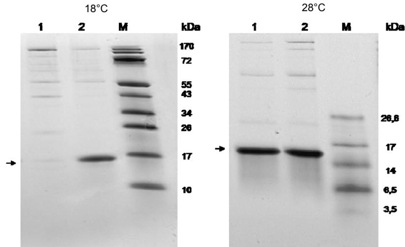
**Fig. 4.** DNA affinity chromatography with *IscB* upstream sequence and proteins from *P. putida* transconjugants. SDS-PAGE of proteins isolated from *P. putida* transconjugants grown at 18 and 28°C, respectively, incubated with *IscB* upstream DNA linked to magnetic beads, and eluted with 1 M NaCl. Lanes: (1) *P. putida* (*IscB*, *IscR*); (2) *P. putida* (*IscB*). The protein band for MvaT (PP1366) as determined by MALDI-TOF MS and peptide mass fingerprint analysis is indicated by the arrow.
