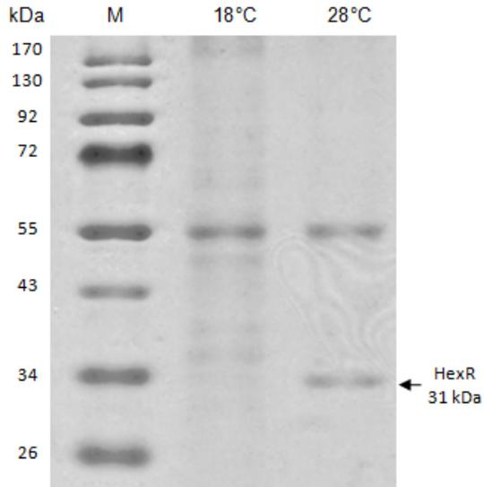
**Figure 5.** SDS-PAGE of proteins isolated from crude protein extracts of *P. syringae* grown at 18°C and 28°C, respectively, using DNA affinity chromatography with the *IscB* upstream region as bait. The arrow indicates a 31-kDa protein found in protein extracts of 28°C-grown cells and identified as HexR by MALDI-TOF MS and peptide mass fingerprint analysis.
